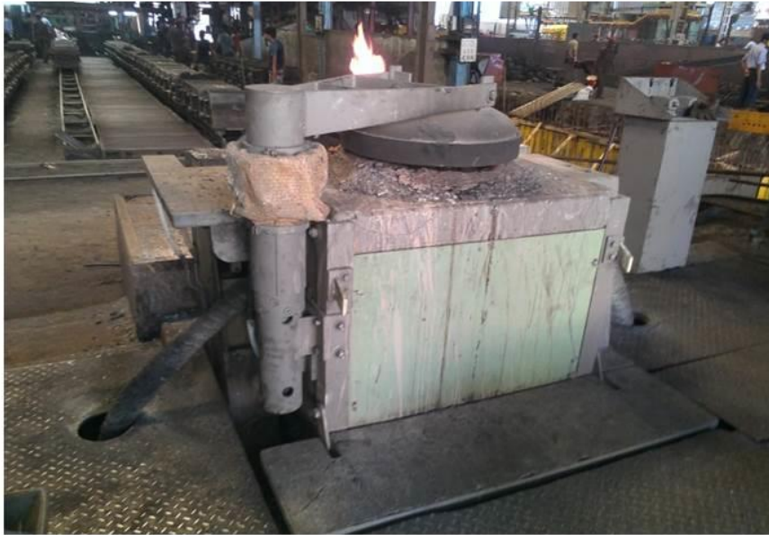
Lid mechanism for induction furnace crucible
